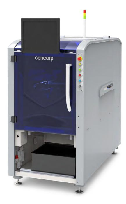
The cencorp Raptor is true high-volume machines designed for high-speed placement of small through-hole components, giving you an excellent return on investment.
