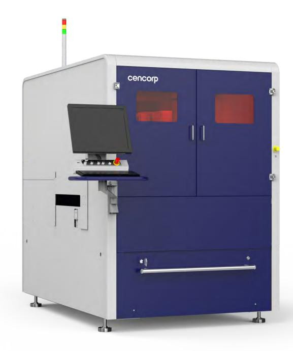
Laser Depaneling Equipment: Cencorp 1300 LR is mainly used in the FPC industries, providing users with simple, fast, consumable free, noncontact, high-precision cutting solutions of any shape. The maximum product processing size can reach 450 \*350 mm.
