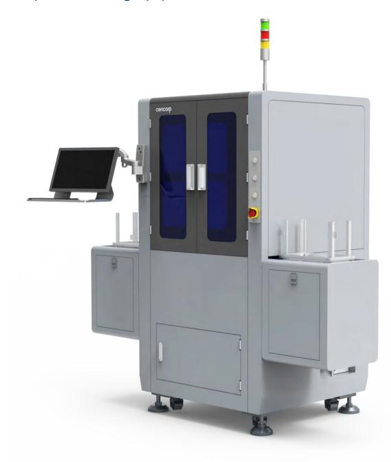
Cencorp 1000 LM SC is mainly used for Semiconductor industry. It can laser mark IC chip of different sizes. The chip carrier can be switched quickly between different products to increase the production flexibility.
